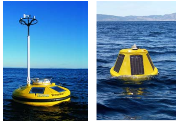
Figure 1: The WAVESCAN heave/pitch/roll metocean data buoy (left) has been used worldwide for directional wave measurements since 1984; The SEAWATCH Mini mk. II (right) is used for coastal and on-site directional wave data collection (for instance, 8 of these buoys form the core of an instrumentation network at the Wave Hub site off the South West of England)
